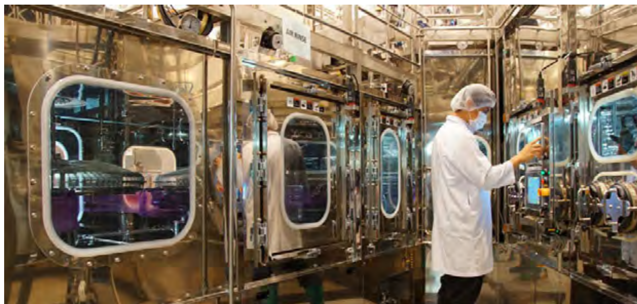
The staff is monitoring the filling machine in the ready-to-drink tea bottling process.
