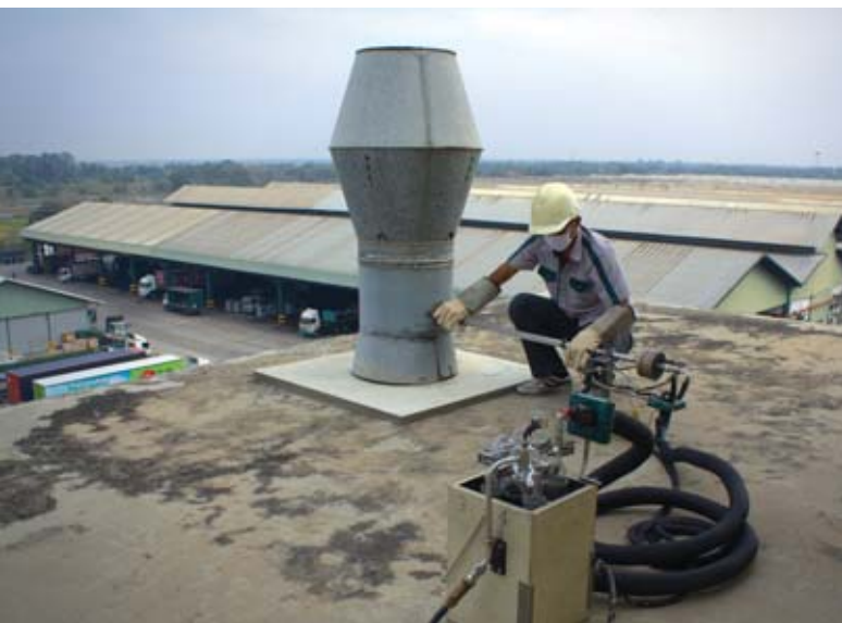
Operator of air pollution control department is measuring air quality at the chimney of Beerthip brewery (1991) Co.,Ltd.
