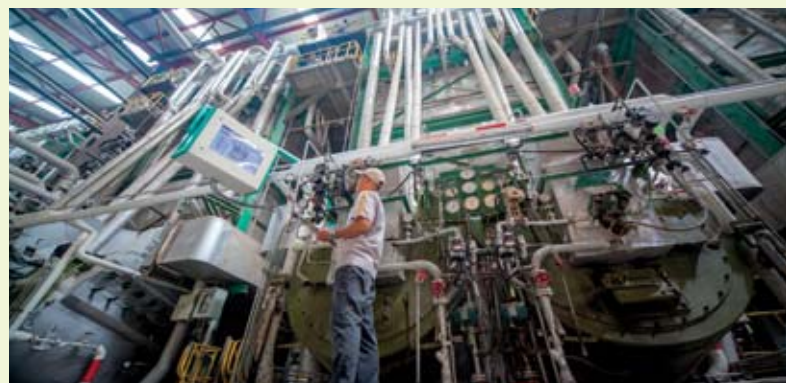
Steam Incinerator fueled by concentrated slop at Sura Bangyikhan Co., Ltd.
